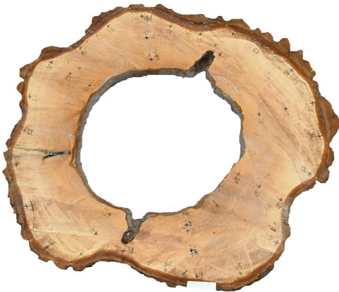
lime tree with central cavity:
